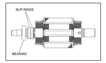
Figure 9. The Rotor Assembly
